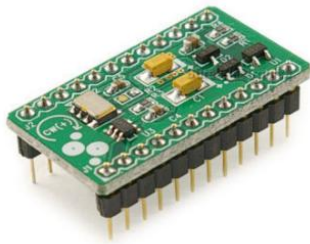
Fig. 14. Piezoelectric gyroscope with XV-3500CB chip used for sensing angular velocities of the helicopter's body.
