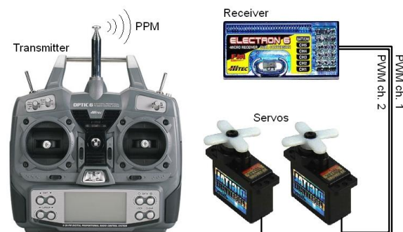
Fig. 3. Communication between the transmitter and receiver through PPM signals and servo control from the receiver through PWM signals.
