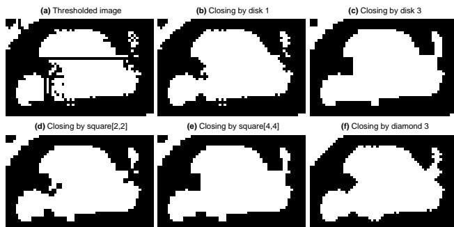
Figure 5. Selected results of closing operation by means of various types of structural element in zoomed cut of an image: (a) Part of thresholded image, (b) Closing by disk size 1, (b) Closing by disk size 3, (d) Closing by square size [2,2], (e) Closing by square size [4,4], (f) Closing by diamond size 3
