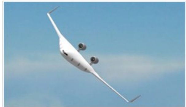
Figure 1 The ACFA 2020 blended-wing-body aircraft
